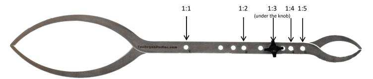
To change scales, simply unscrew the knob and move the stud to the desired set of matching holes and retighten the stud and knob.
